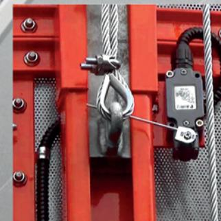
The auger system and the screens will be lifted up or down just with the pression of a button. Furthermore an electronic safety device grants that the controlled parts move only when requested.
