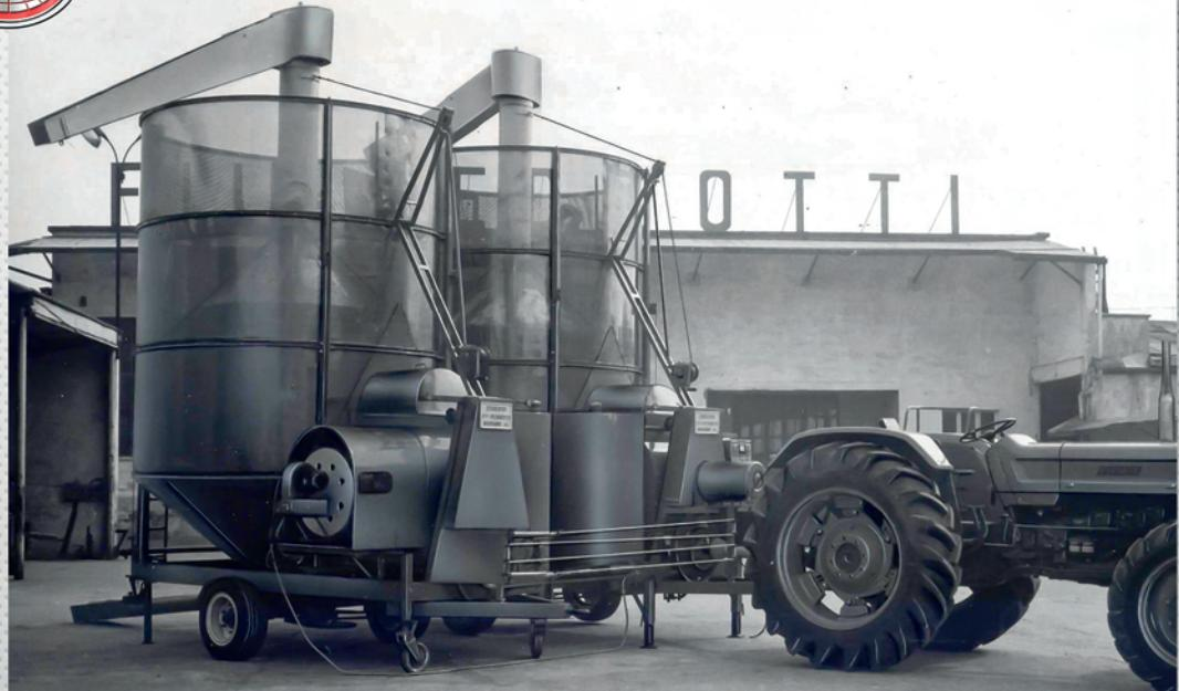
THE FIRST RETRACTABLE MOBILE GRAIN DRYERS
